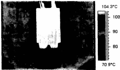
Figure 6b: IR temperature gradients across top surface of vapour chamber at 2000W
