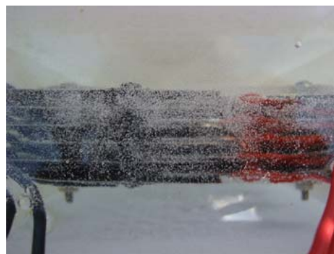
Figure 6. Photograph of PV-driven gas bubble evolution off of an electrode array consisting of four double-sided anodes with matching stainless steel cathodes.
