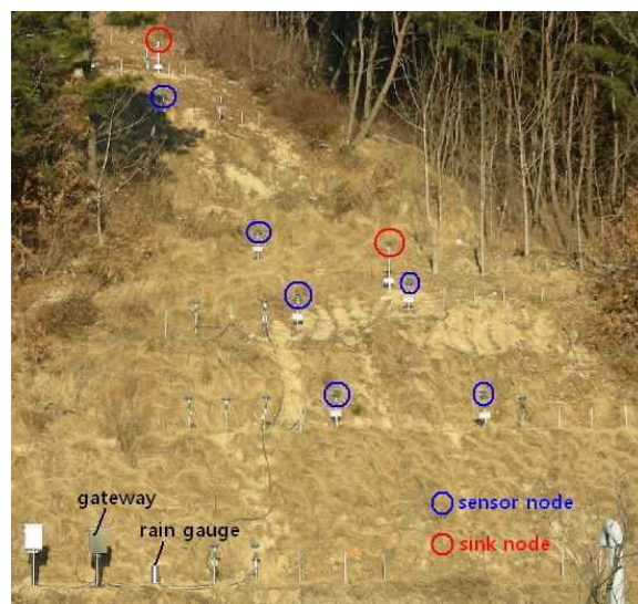
Figure 6: System Installation Site
