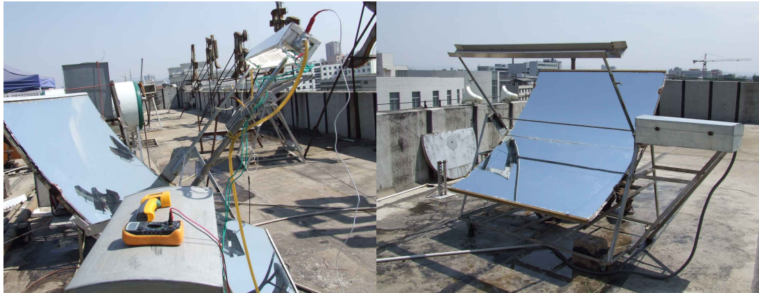
Fig.2 Photographs of the trough concentrating PV/T system
