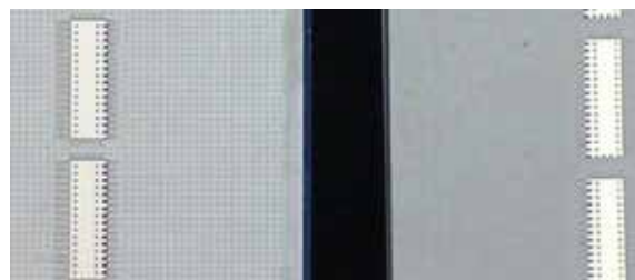
Figure 4: Comparison photo of the back surface field of pointed contact solar cells (left) with the conventional full Al BSF solar cell (right)
