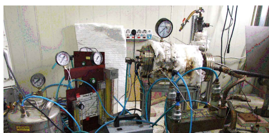
Figure 3: The reformer with fuel tank under pressure, flow meter & gas sampling pump.
