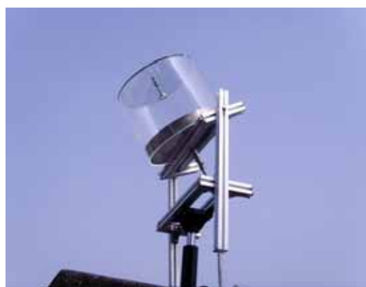
Figure 4: A fiber optic solar daylighting system with one concentrator unit.
