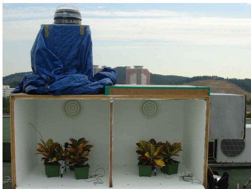
Fig. 4. Experiment chambers installed on the roof (with the front cover opened)
