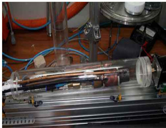
Figure 3: ZnO coating on the acrylic tube surface using a plasmatron.
