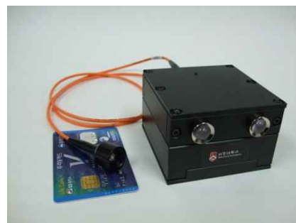
Fig. 4. (a) Structure of hydrogen optical sensor (b) The photograph of hydrogen optical sensor
