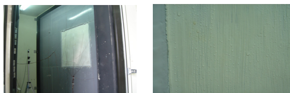
Figure 2: Installation of test object and phenomenon of dewing occurrence
