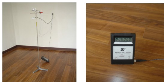
Figure 3: Radon measurement of mock-up test building
