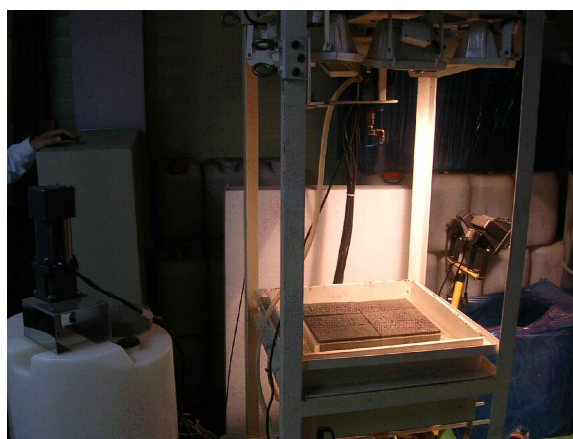
Figure 4: Water quality purification test of bottom ash block
