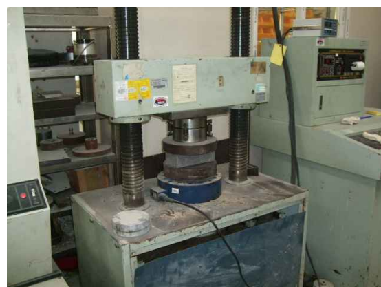
Figure 2: Compressive strength test
