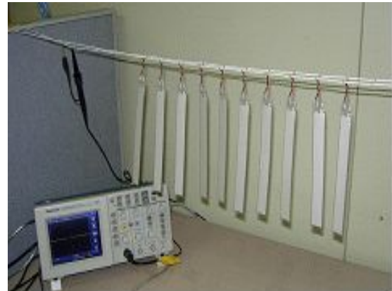
Figure 5: Experimental setup to measure any electric current from a series of piezofilm connected in parallel
