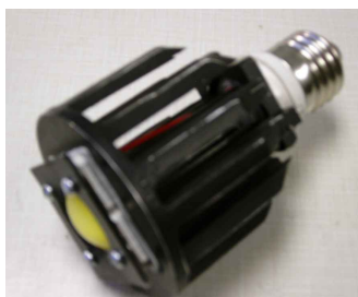
Figure 2: Pin-fin array developed at the University of Utah for LED cooling.
