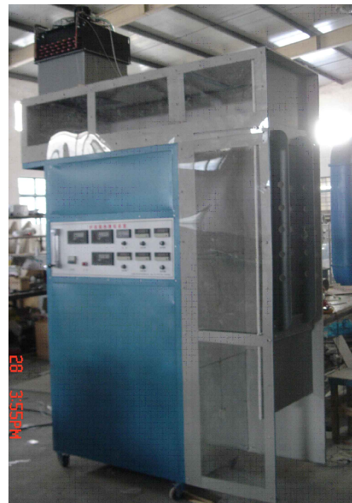
Figure 2: Heat recovery experimental device of furnace wall
