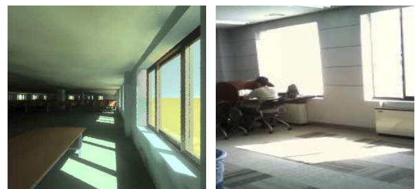
Figure4: Comparison of direct sun penetrations
