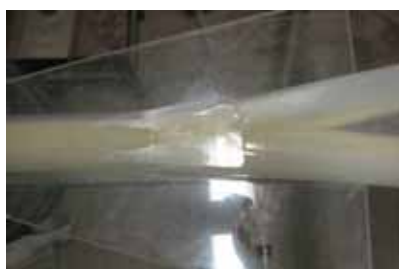
Figure 3: Flow style of the branch pipe with the angle \beta = 10^\circ
