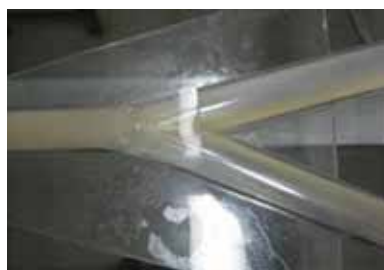
Figure 4: Flow style of the branch pipe with the angle \beta = 30^\circ
