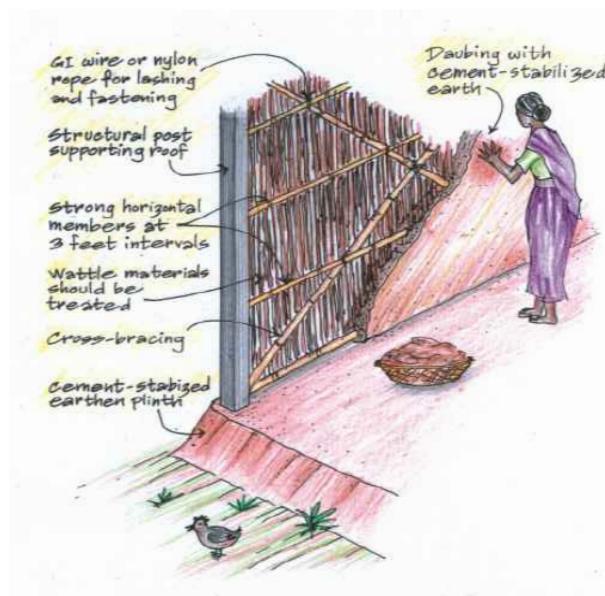
Figure 5: wattle-and-daub construction [3].
